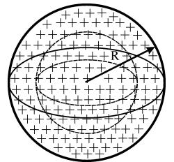
electrical charge uniform distributed in the entire volume. The total charge is denoted by Q and the sphere radius by R.
